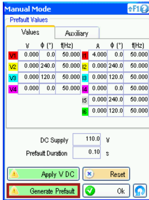
Figure 7 How I set the Prefault that managed to drive the current thru the Relay
