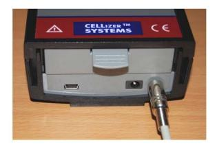
For security reasons, all interfaces are placed behind a plastic cover. The rechargeable battery pack can easily be replaced.
