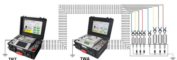
Connecting TRT400 and TWA40D to a three-phase transformer
