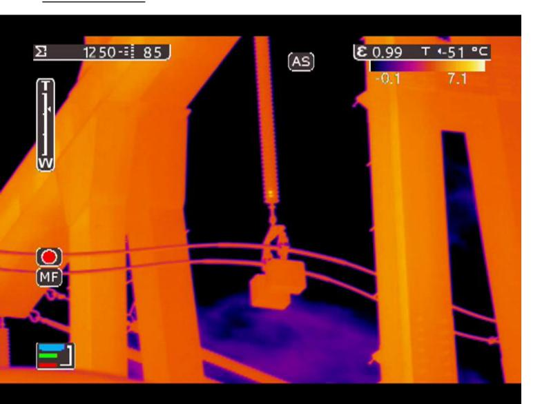
The hotspot is not at the end fitting, but further up the shaft, at the 2nd / 3rd shed.
